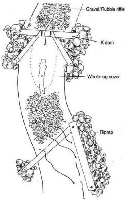
*Hypothetical plan view of a structure installed in reaches of a high-gradient stream.*
